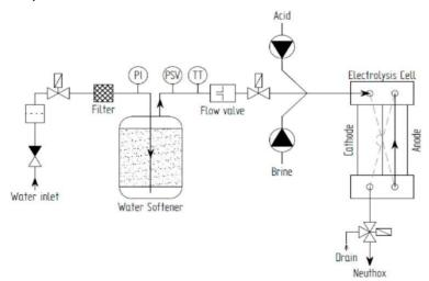
What makes Neuthox special is that all the liquid is exposed to both sides of the membrane. First the liquid passes through the negative cathode and then through the positive anode. The flow is never divided during this process, therefore the risk creating chlorine gas is eliminated. Additionally, the final product is approximately 8.3 pH - close to neutral pH.
